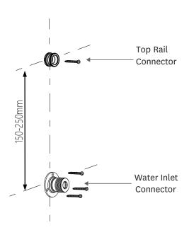
Screw the bottom rail connector to a wall stud making sure it is vertically in line with the top rail connector. Maximum centre distance between the top and bottom shower connections is 250mm.
