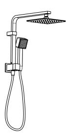
Make sure a washer is in both ends of the hose. Screw hose onto lower outlet on rail, attach handset and place firmly in holder. Tilt and rotate head to the desired position.
