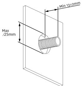
Install a ½" male threaded connection at the recommended height on wall, ensuring that a minimum of 13±2mm of thread protrudes past the finished wall.
