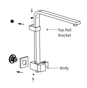
Check the grub screws are woundtou. Push the body onto the top rail connectors until it is gainst wall. Secure with grub screws.
